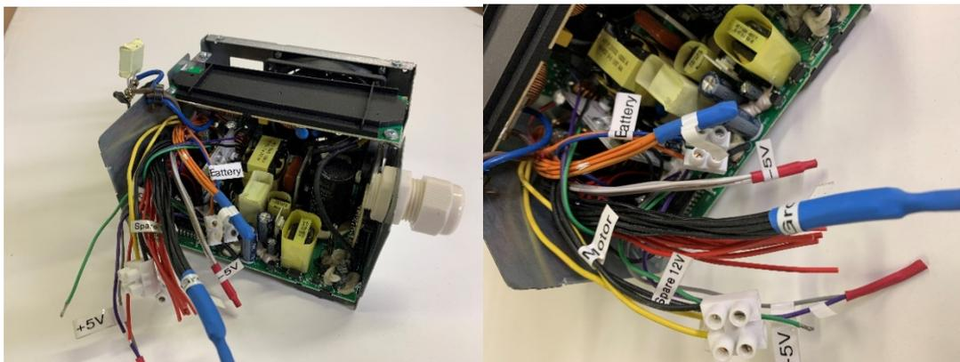
Fig: 3) Picture showing sample opened PC power supply with labelled cables
