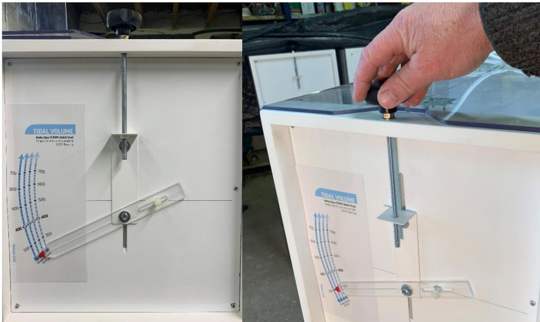
Fig: 8) Tidal volume handwheel/pointer adjustment range for different Peep pressures
