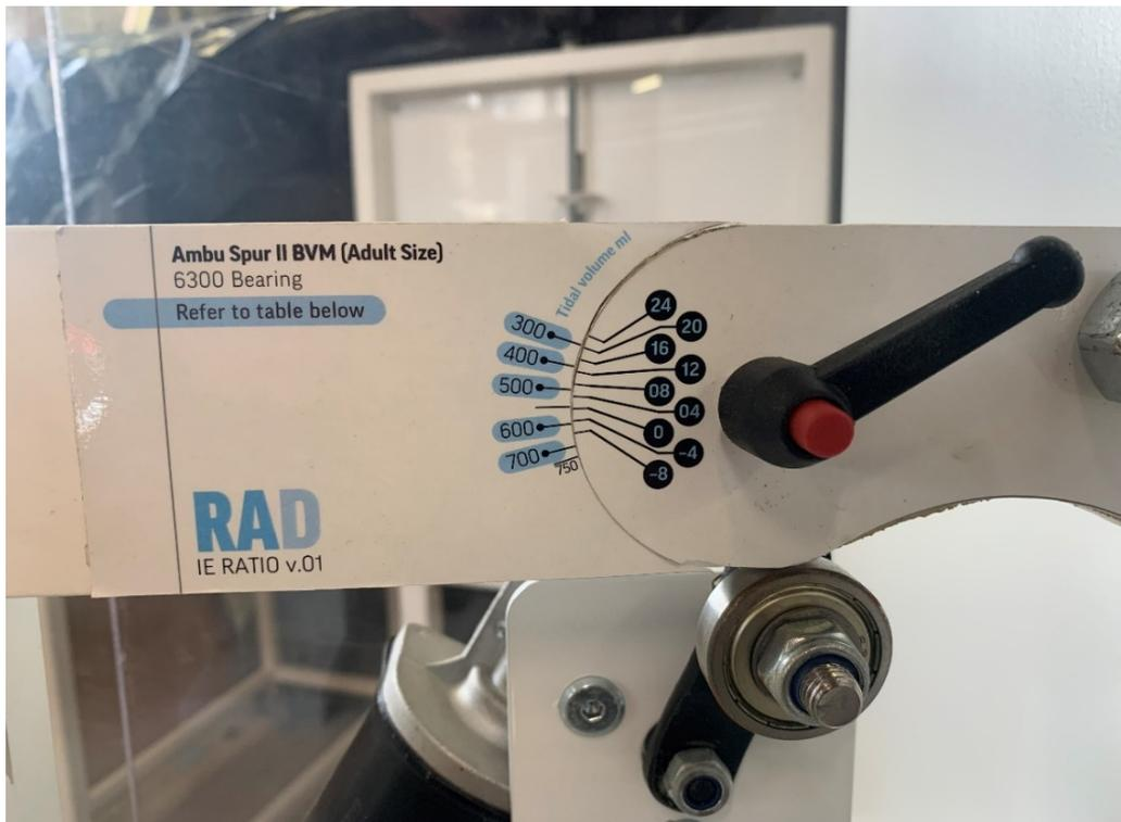
Fig: 9) Adjustment scale on actuator arm
