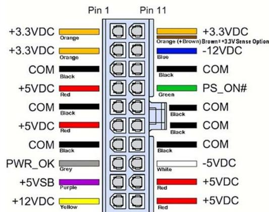
Fig: 6) Output voltages of a typical personal computer power supply
