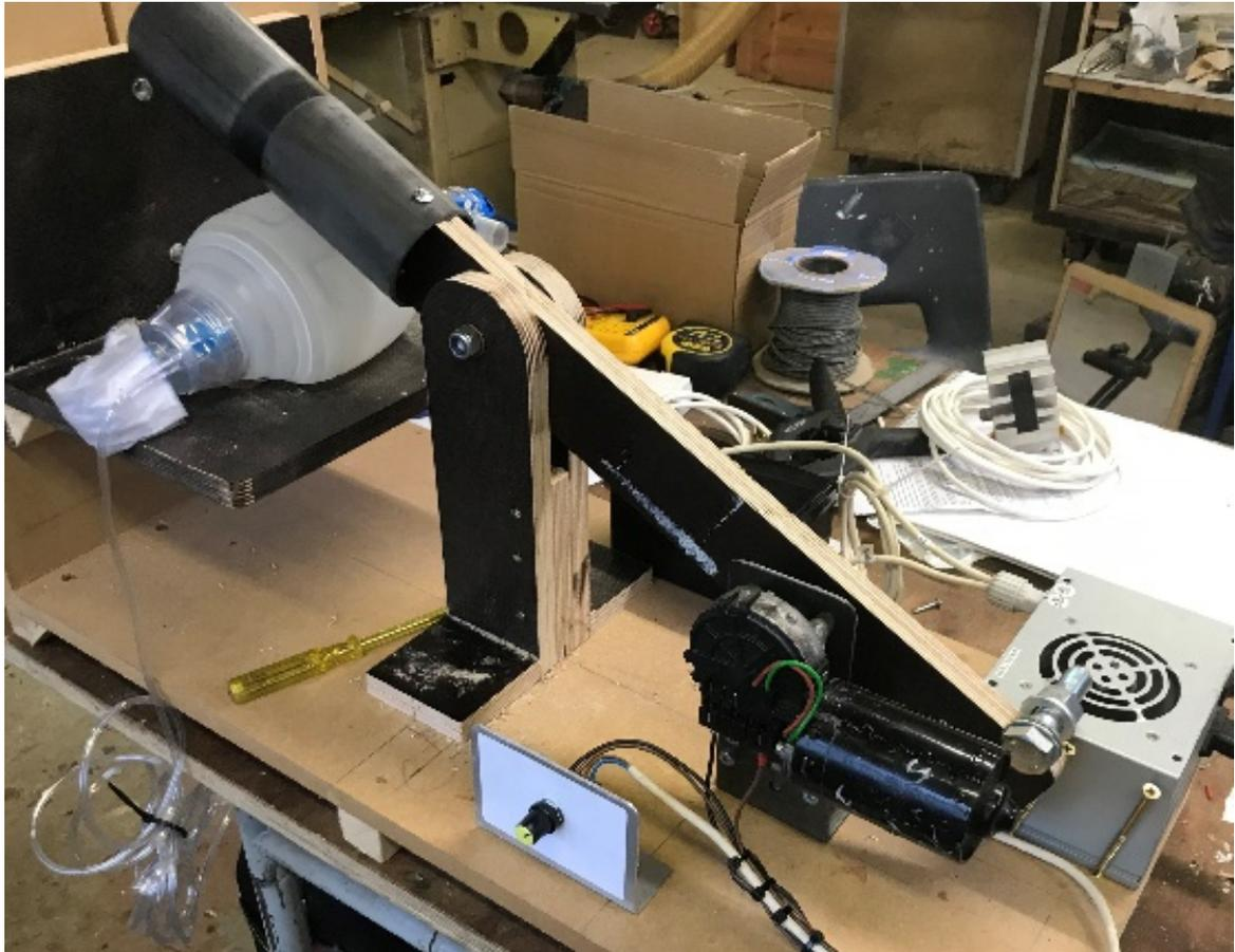
*Fig: 7) Actuator arm on basic prototype*
