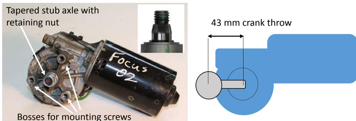
Fig: 2) Typical Bosch Wiper Motor – Note mounting screw bosses and crank/spigot arrangement
